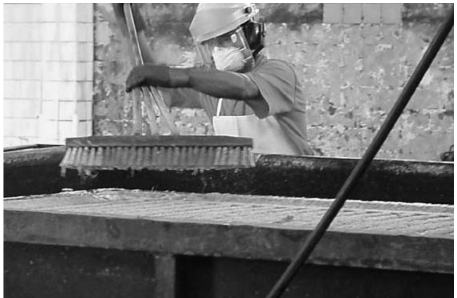
Figure 7—After immersion and impregnation, worker “brushes” asbestos diaphragm surface in order to smooth it, wearing an improper respirator.
